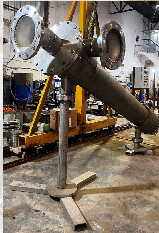
HYDRO CYCLONE SEPERATOR
