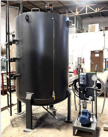
OIL STORAGE TANKS WITH OIL TRANSFER TROLLEY
