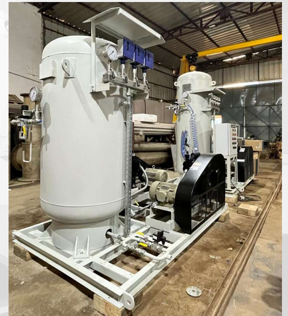
SKID MOUNTED COMPRESSED AIR SYSTEMS
