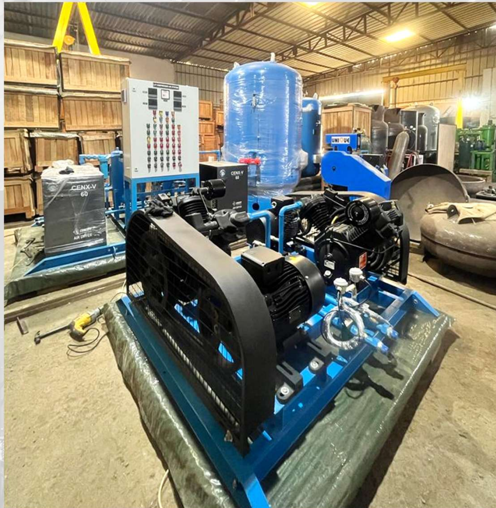
DUAL COMPRESSOR AIR SYSTEM WITH AIR DRYERS & 2 TANKS [ 3000 Ltrs. & 1000 Ltrs.]
