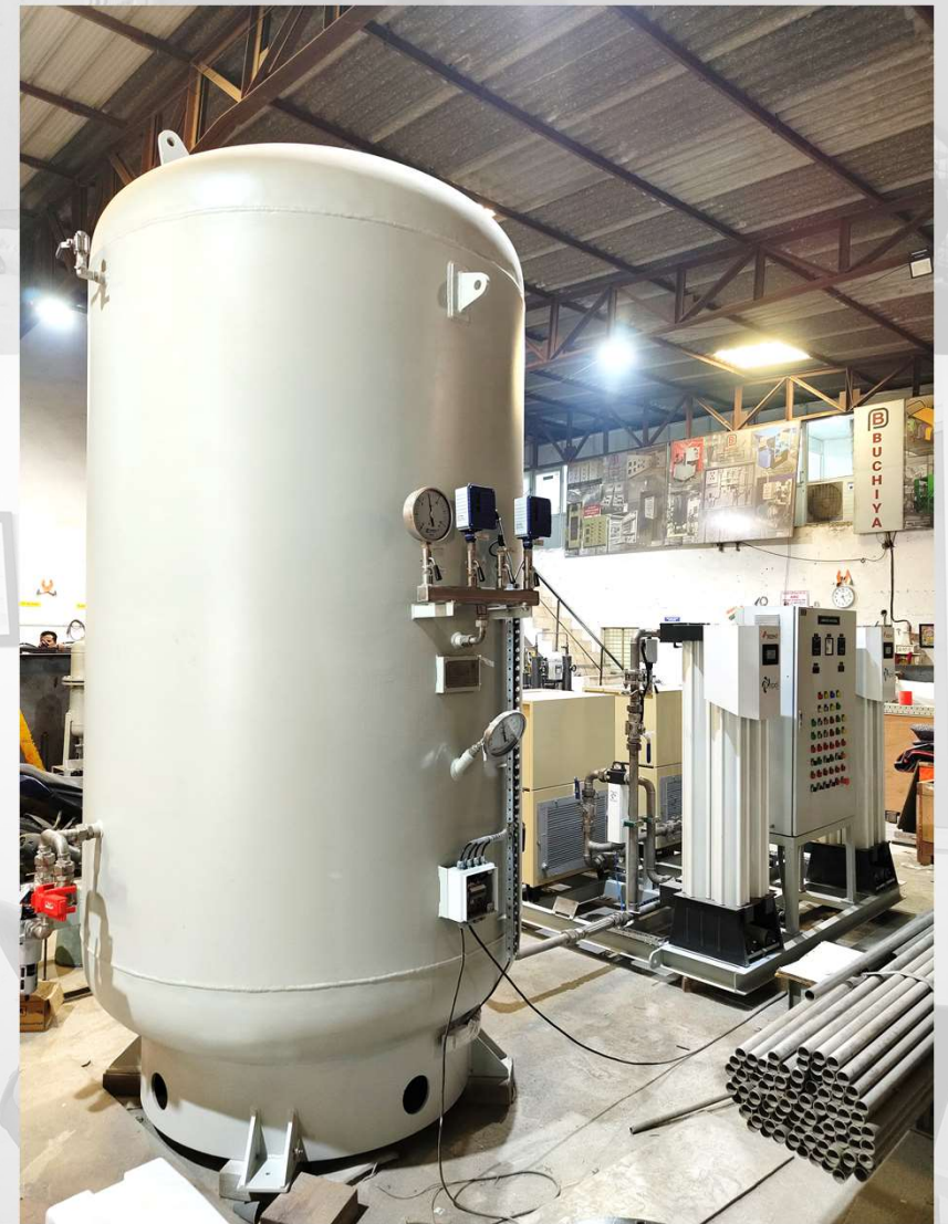
DUAL SCREW COMPRESSOR AIR SYSTEM WITH AIR DRYERS, AFTER COOLER & TANK (5000 Ltrs)
