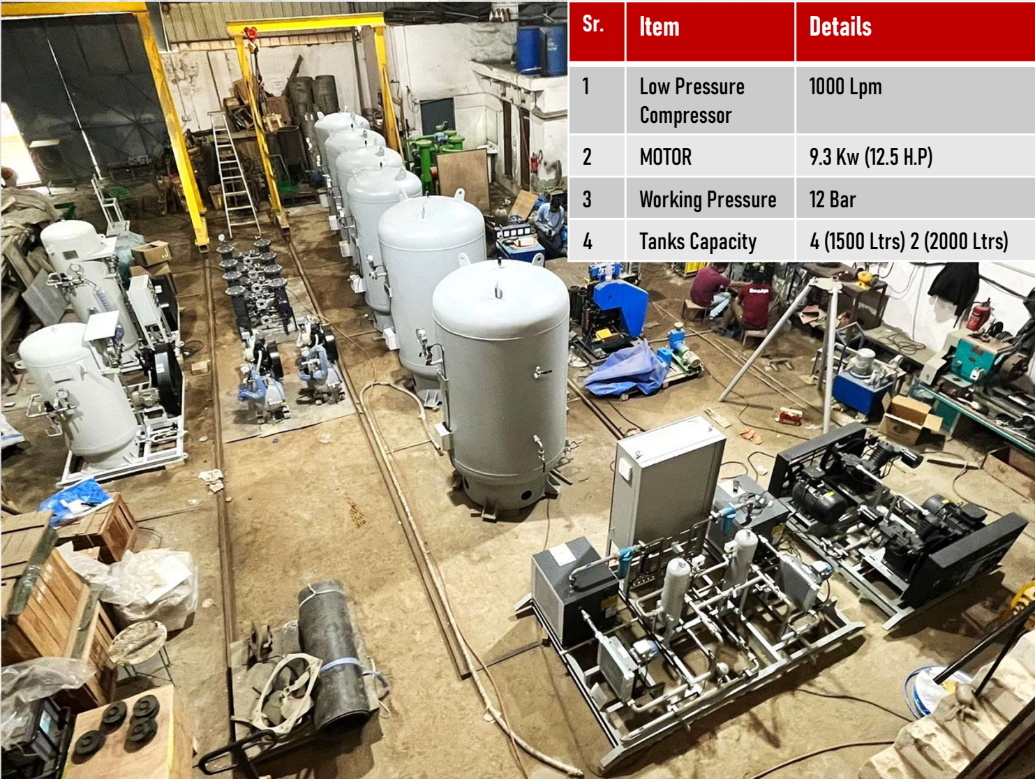
DUAL COMPRESSOR AIR SYSTEM WITH AIR DRYERS, AFTER COOLER & 6 TANKS
